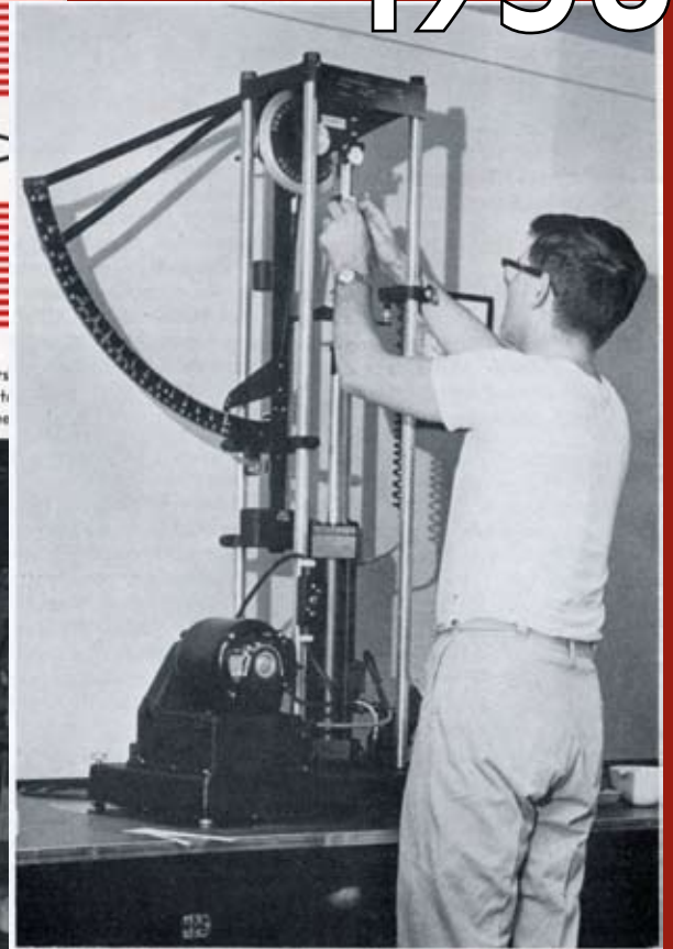
Small sheets of paper made in the laboratory are tested on the Tensile Strength Tester under rigid conditions demanded by the industry. This testing is done in a humidity and temperature controlled room.
